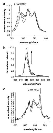
**Figure 10.** Selected europium emission spectra for  $[\text{EuL}^{1c}]^{4+}$  (1 mM, 295 K, H<sub>2</sub>O,  $\lambda_{\text{exc}} = 365$  nm) in the presence of increasing concentrations of NaHCO<sub>3</sub> (0, 2.1, 4.2, 8.3, 19 mM), highlighting the large increase in intensity of the  $\Delta J = 2$  manifold (b) and the change in the form of emission of the  $\Delta J = 1$  and = 4 bands (a and c, respectively).
